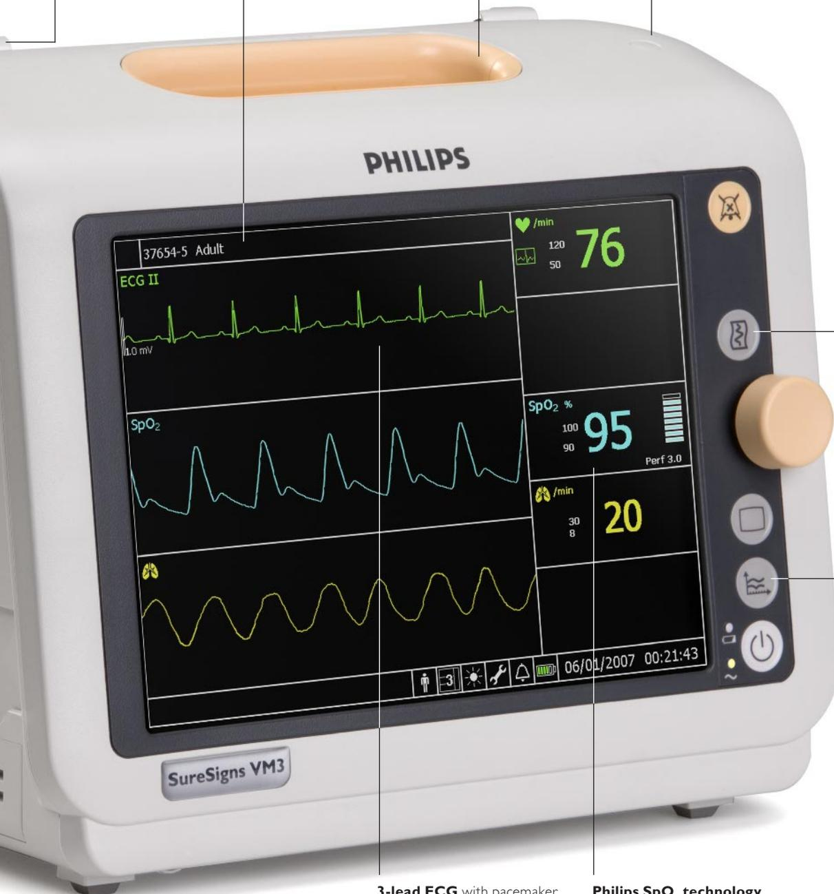
**3-lead ECG** with pacemaker detection, including a "leads off" indicator.
